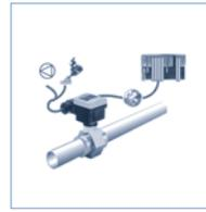
Monitoring of min./max. levels of temperature in a running process (compact INLINE control)
